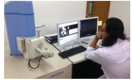
Scanning Electron Microscope (SEM) observation by researcher, the SEM including X-ray energy Dispersive Spectrometry system use for observing mineral and structure of the mineral, including element map of the samples.
